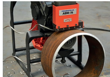
Oval workpiece and pipe beveling
