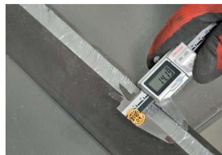
Maximum bevel width up to 14 mm
