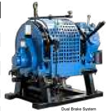
Dual Brake System Automatic & Inching Brake
