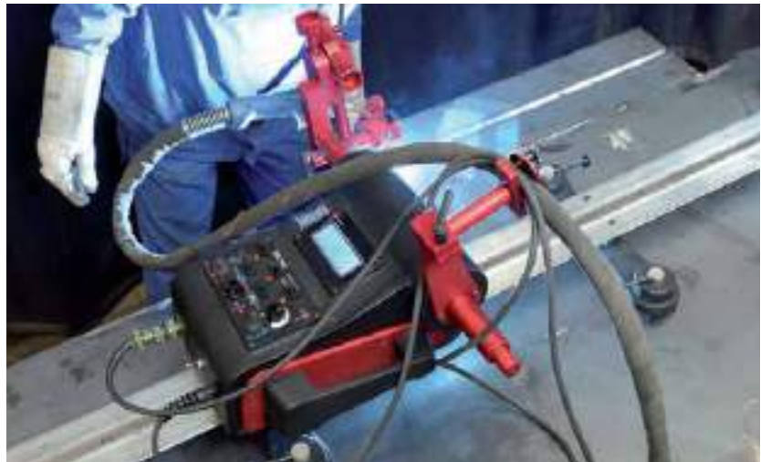
RAIL BULL TRACK WELDING CARRIAGE WITH OSCILLATOR
