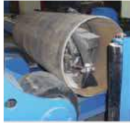
Small-diameter pipes welding head
