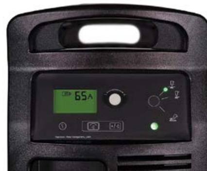
The SmartSYNC® torch automatically adjusts the amperage and chooses the correct cutting or gouging mode.
