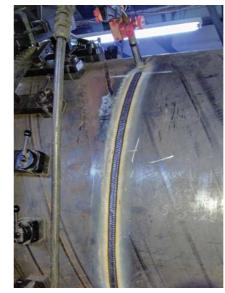
An application trial being done at Renttech's Alrode premises. The root weld is being done using the Böhler Ecospark 420 (ER70S-6) solid wire and the Wiseroot function on a Kemppi welding machine. The fill and cap was then done using is the Bohler Diamondspark 46RC (E71T-1M) flux-cored wire using a Promotech Rail Titan welding and cutting tractor.
